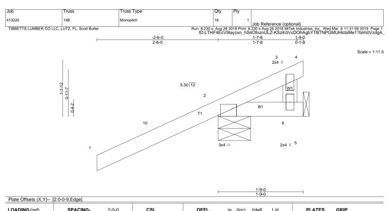
LOADING (psf) SPACING-CSI. DEFL. I/d **PLATES** 2-0-0 (loc) I/defI Plate Grip DOL 1.25 0.50 TCLL 20.0 TC Vert(LL) 0.00 >999 360 MT20 TCDL 1.25 ВС 15.0 Lumber DOL 0.14 Vert(CT) 0.00 9 >999 240 **BCLL** 0.0 Rep Stress Incr YES WB 0.00 Horz(CT) 0.00 2 n/a n/a **BCDL** 10.0 Code FBC2017/TPI2014 Matrix-MP Wind(LL) -0.00 9 >999 240 Weight: 10 lb
