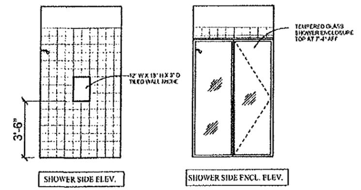
BATHROOM TUB ELEVATIONS 'B-B'
