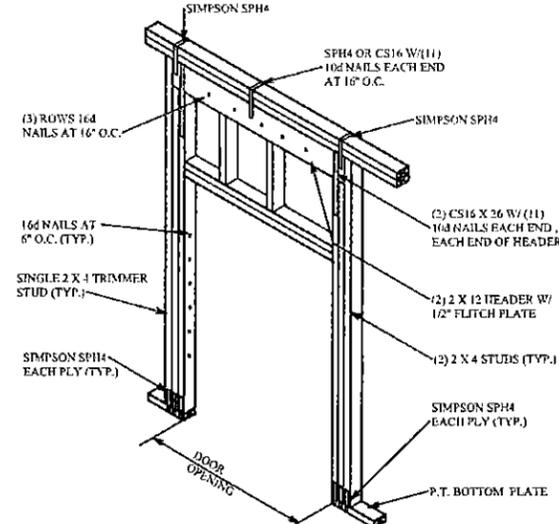
**TYPICAL LOAD BEARING HEADER DETAIL**
